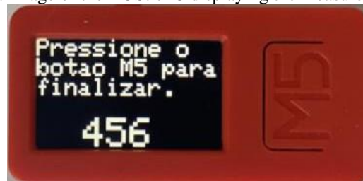
Figure 04: Image of the M5StickC displaying the measurement value.
