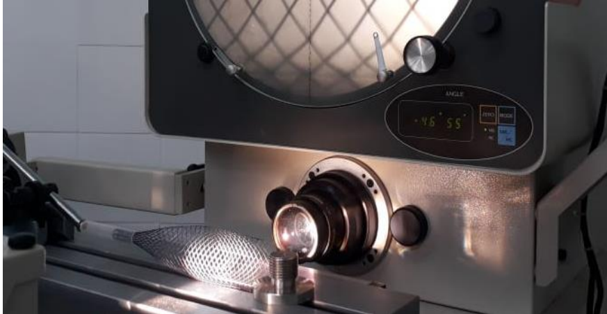
Figure 2 - Setup of the experiment for measuring X and Y, with the Mitutoyo PJ-A3000 Profile Projector
