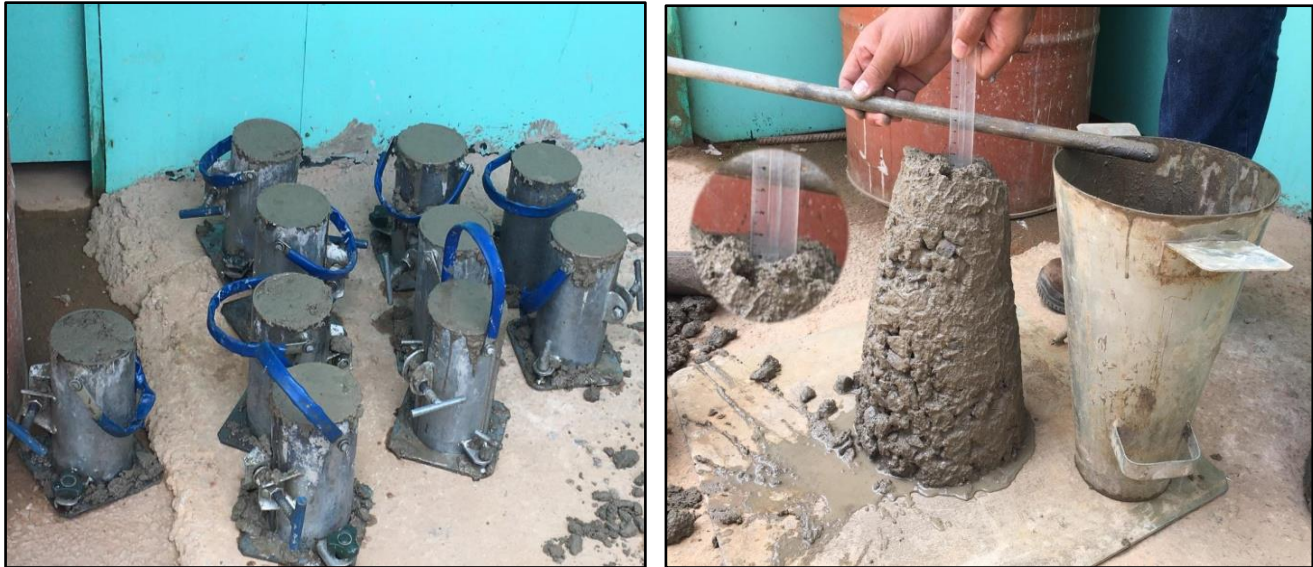
Figure 10 a) Fabrication of specimens and b) Shakeout test
