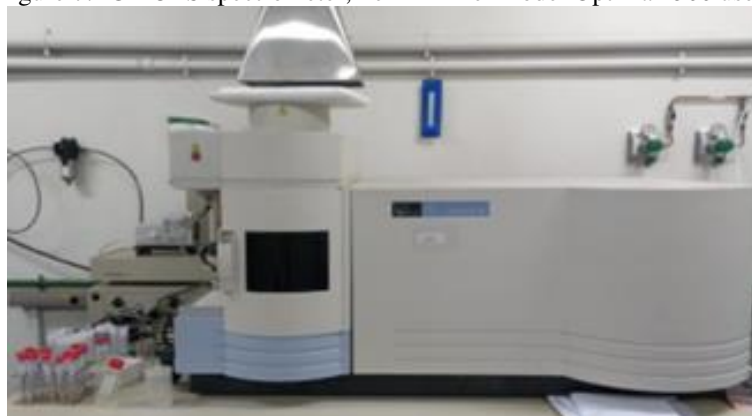
Figure 7: ICP-OES spectrometer, PerkinElmer model Optima 4300 used.
