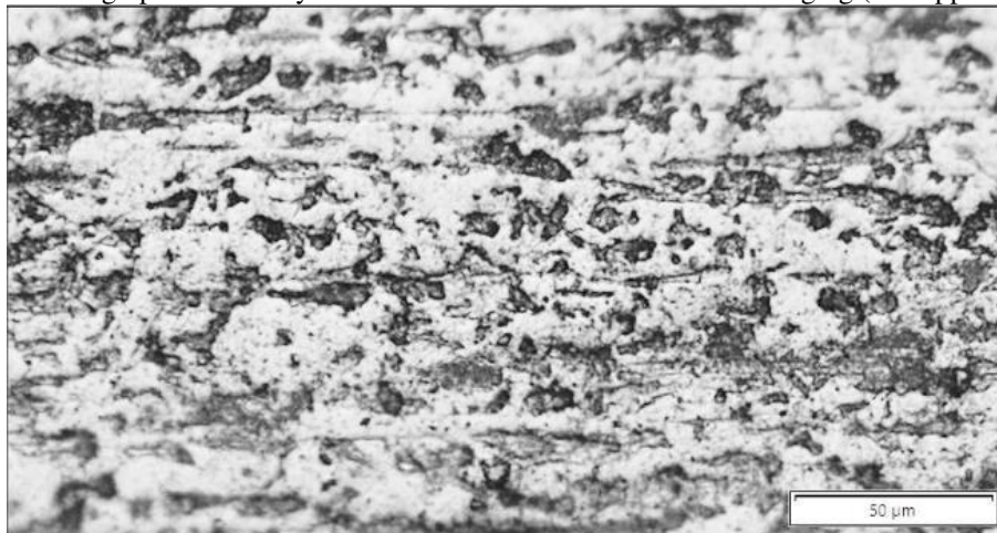
Figure 9 – Micrograph of the alloy submitted to solubilization and 0.5 h of aging (20x approximation).
