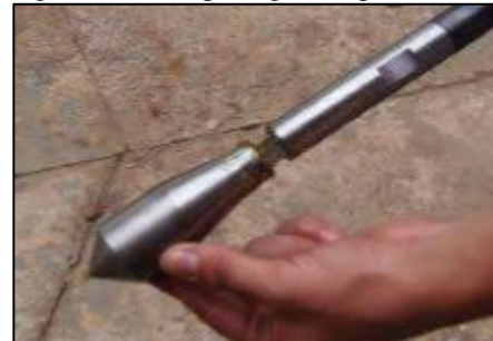
Figure 2. DPL tip for ground penetration.
