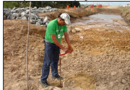
Figure 9. Preparation for carrying out the “vane-test”.
