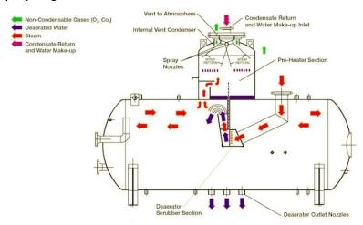
Pressure degassers, whether spray or tray, are used in any industry where the heat transfer fluid is water-vapor and this water must be reduced in chemical substances intended for the elimination of gases for reasons of size, function, etc. The use of spray type in practice has been carried out for process plants where the size of the equipment is relatively important.
