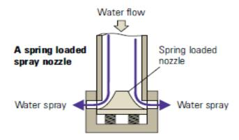
Figure 2. It gives in more detail what the upper area of a deaeration tower is like, in which water is atomized and a current of vapor creates an atmosphere responsible for raising the temperature of the returned condensate and the incoming make-up water.
