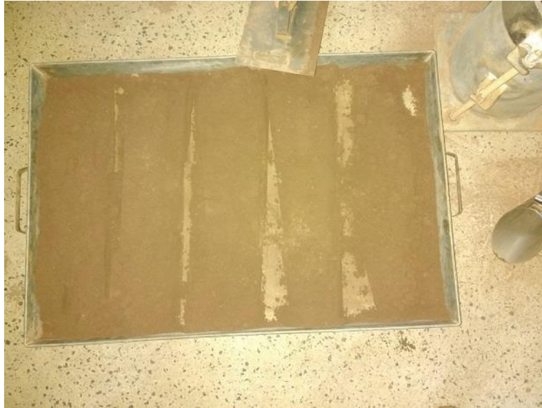
Figure 3.2 – Separation of the sample into five portions.
