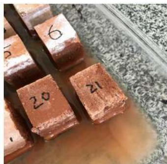
Figure 9 - Loss of mass of RTM-based mortars.
