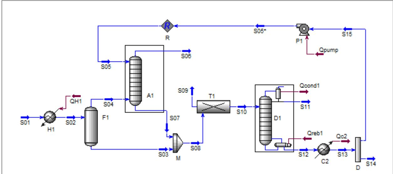
Figure A.2 – VR diagram in the UniSim interface.
