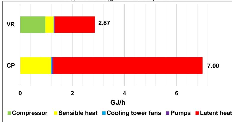
As demonstrated in this work and in Figueiredo et al. [23], sensible heat is critical in the energetic evaluation, accounting for over 17% of the total energy required in the boiler for the MCB separation process. Many studies do not consider this type of heat since, in simulation software, credit is only taken for the latent heat. Consequently, deviations in the energy analysis are found, leading to errors that reflect in the acquisition and purchase of utilities.
