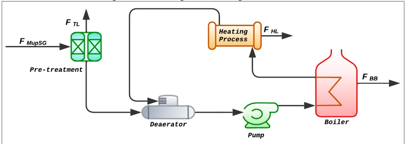
Likewise, in the CS, SG has losses to be taken into account, such as treatment ( $F_{TL}$ ) and heating losses ( $F_{HL}$ ) as well as boiler blowdown ( $F_{BB}$ ). Hence, another make-up stream ( $F_{MupSG}$ ) is added.
