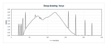
Note that in figure 5 there are some spikes on the deep drawing profile, that is some noises generated during the deep drawing operation.
