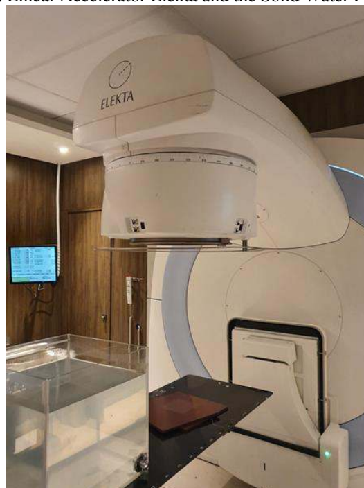
Fig. 1. Linear Accelerator Elekta and the Solid Water Phantom.
