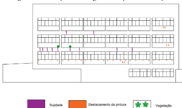
Figure 16 - Map of damage to the posterior façade
