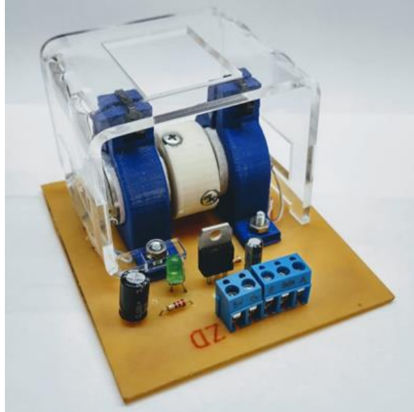
Figure 3: Motor-tacoker module used to validate the proposed approach.
