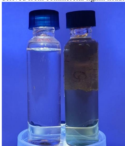
Figure 1. Luminescence of GQD solution derived from commercial lignin irradiated with UV LED 365 nm before dialysis.
