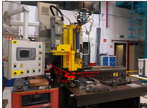
Figure 5: FSW LEGIO 3UL - ESAB® machine
