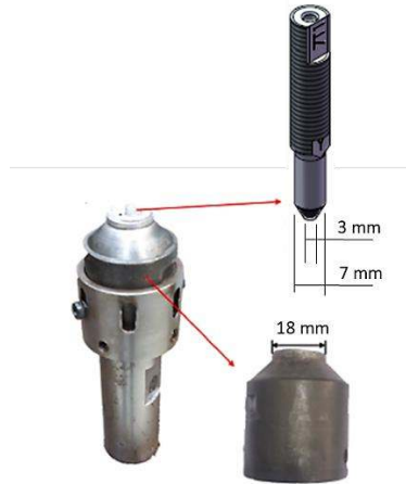
Figure 22: FSW tooling
