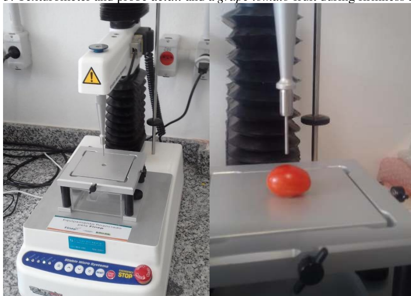
Figure 3: Texturometer and probe detail and a grape tomato fruit during firmness analysis.
