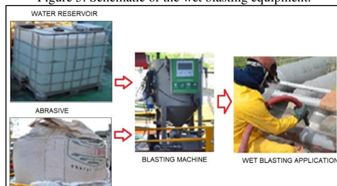
Figure 5: Schematic of the wet blasting equipment.
