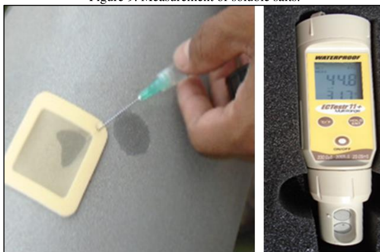
Figure 9: Measurement of soluble salts.
