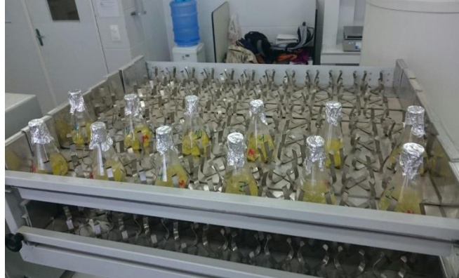
Figure 5 – Shaking of mixture on shake table, under 130 rpm.
