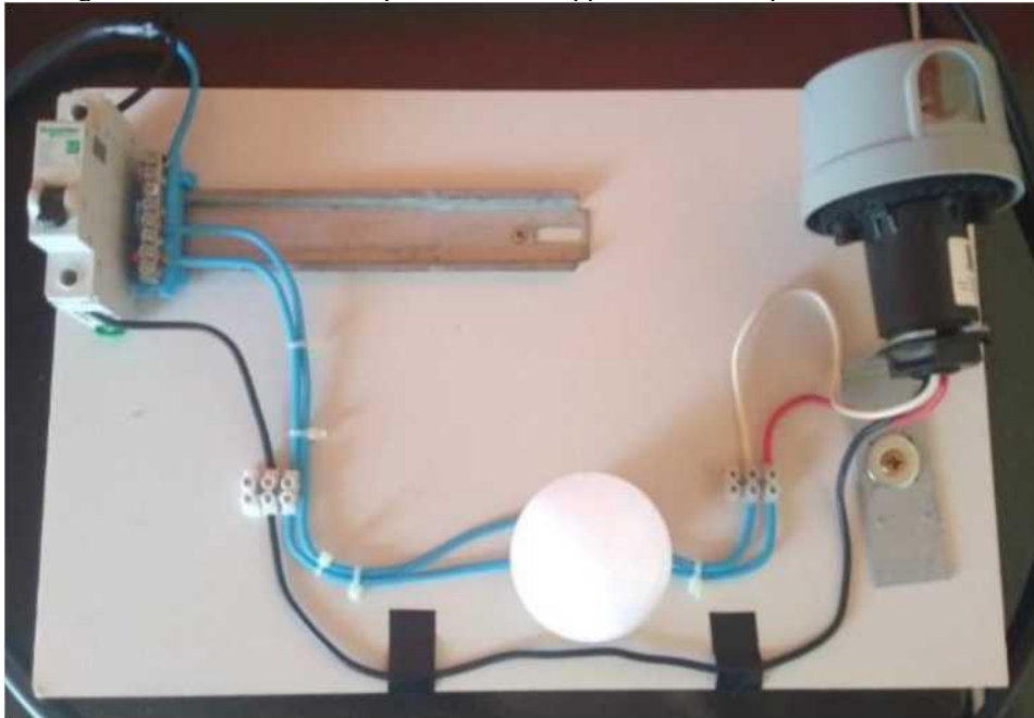
Figure 1 - Demonstration experiment of an application of the photoelectric effect
