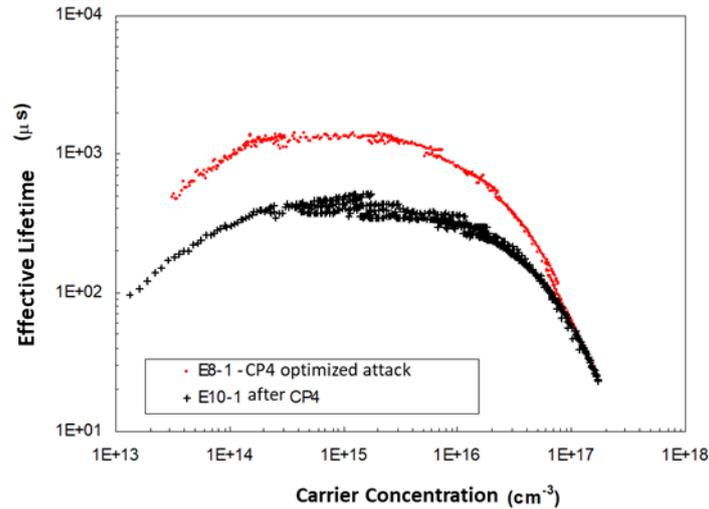
After this measurement, the sample was submitted to a pre-deposition of phosphorus at  $850^\circ\text{C}$ , resulting in a leaf resistance of  $1.4\text{k}\Omega/\square$ , followed by removal of PSG in HF and redistribution of phosphorus/passivating oxidation in chlorinated environment (TCA) at  $1050^\circ\text{C}$ . An  $R_\square = 400\Omega/\square$  was obtained under an oxide with a thickness of  $226\text{nm}$ .
