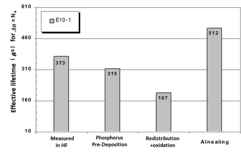
As expected, a decrease in the value of the effective lifetime can be observed along the stages of pre-deposition and redistribution of phosphorus in relation to the initial measure, with passivation in HF.
