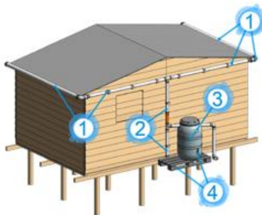
Figure 2: Rainwater capture system for ceiling emergency houses: 1) collection and conduct system, 2) filtering system, 3) reservoir and 4) necessary accessories. (Ceiling, 2018).
