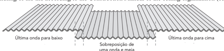
Figure 6: Handling of the tile according to the Construction Manual of the ceiling organization (ceiling, 2017)
