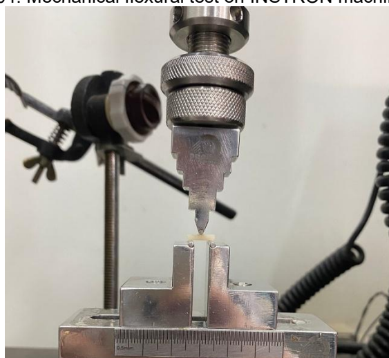
Image 04: Mechanical flexural test on INSTRON machine - 4411
