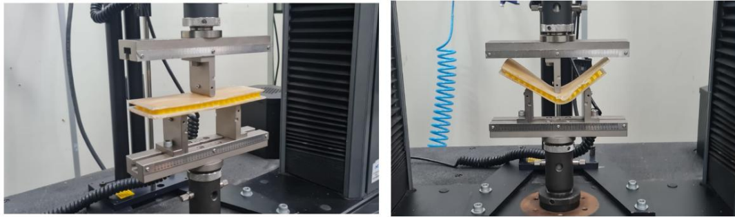
Figure 10: Three-point flexure test of specimen 2
