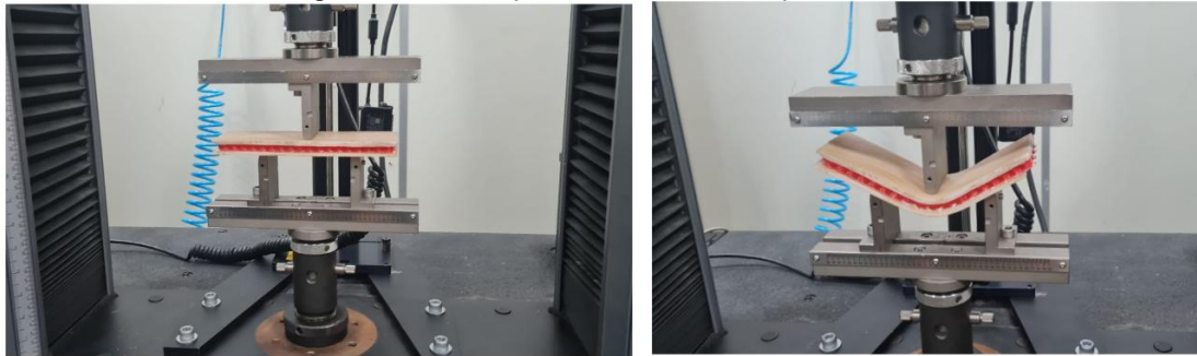
Figure 10: Three-point flexure test of specimen 2
