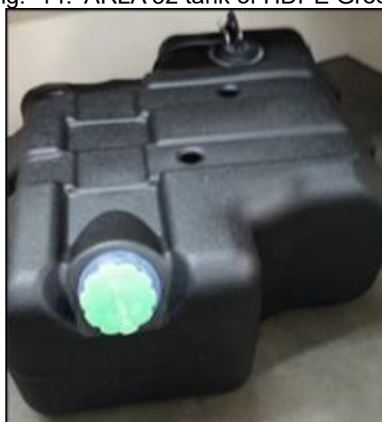
Fig. 14. ARLA 32 tank of HDPE Green.
