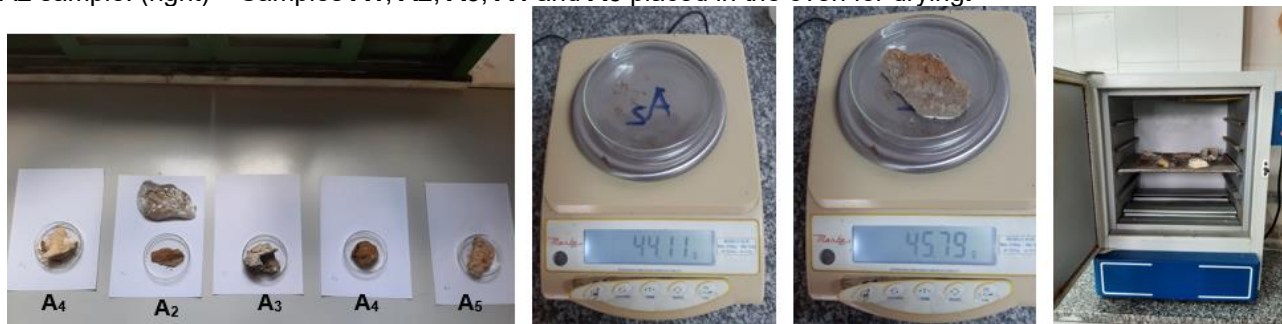
Figure 14: (left) - Sample preparation for visual observation and moisture analysis. (center) – Weighing of the A2 sample. (right) – Samples A1 , A2 , A3 , A4 and A5 placed in the oven for drying.
