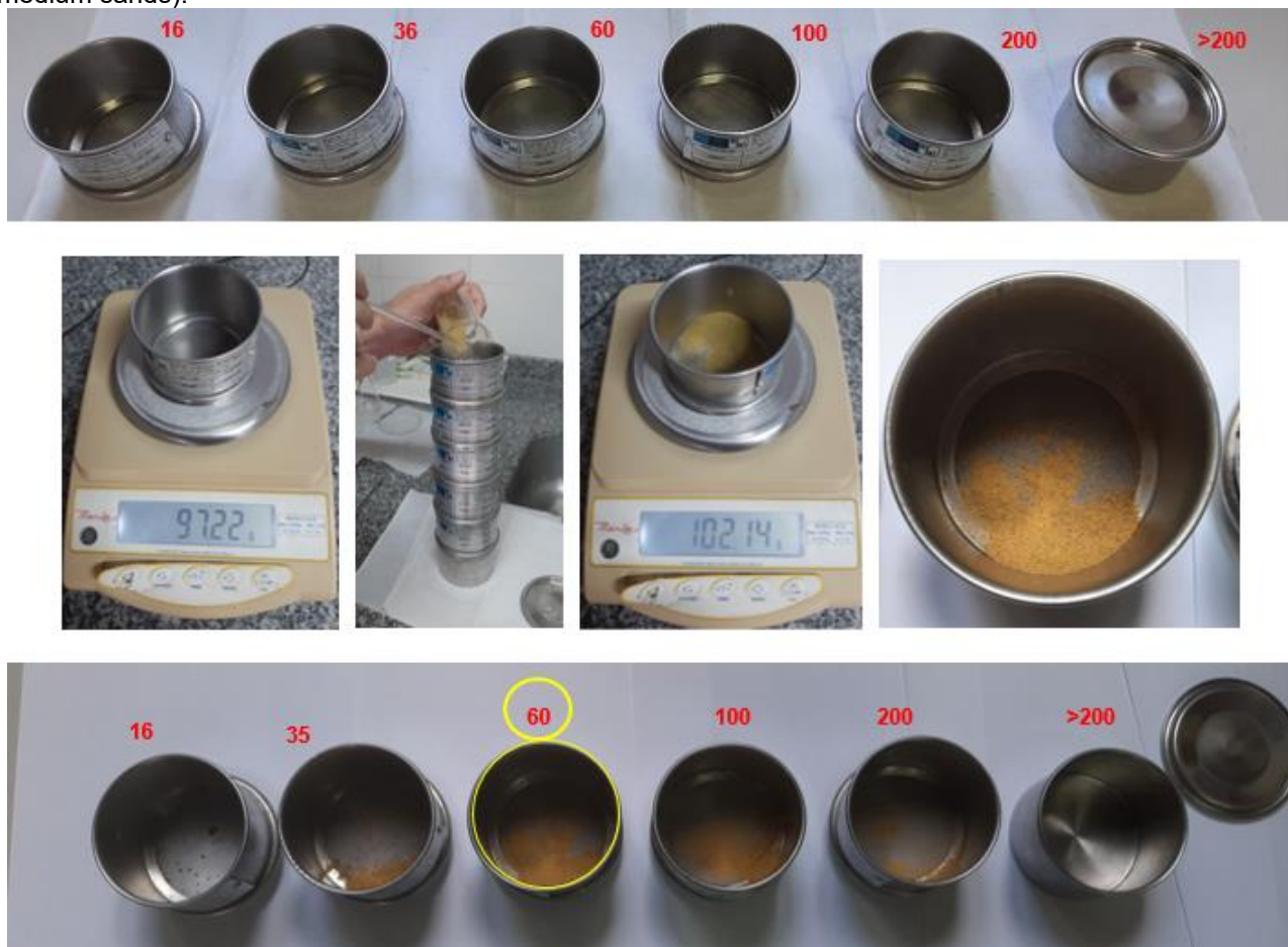
Figure 19: (above) – Sieves of meshes 16, 35, 60, 100, 200 and >200. (center from left to right) • Sieve mesh 35. Placing the beaker thickets for manual stirring for 5 minutes. Sieve weighing 60 + retained material. Sieve 60 with retained material (the one with the highest retained weight). (below) – 16 mesh sieves; 35; 60; 100; 200 and >200 after manual stirring with retained material (in yellow the mesh that retained the most material - medium sands).
