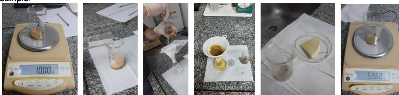
Figure 18: (from left to right) – Weighing of the A4 sample after being distorted for trace testing. Attack with hydrochloric attaché to separate the coarse from the fine (digestion). Filtering of the A4 Sample after acid attack. Result of the separation of the coarse from the fine of the A4 sample. Coarse (beaker) and fine (filter paper) after drying in the oven for 24 hours of the A4 sample. Result of weighing the coarse of the A4 sample.
