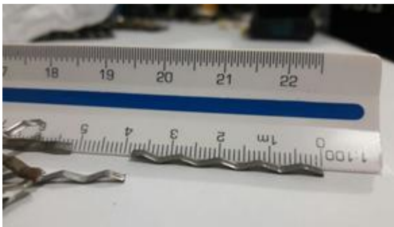
Figure 6 Crimped fiber used in CRFA
